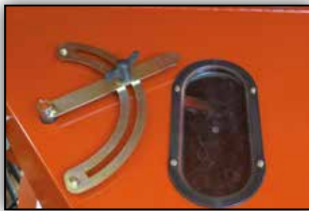
An electronic low level sensor, adjustable from outside the hopper, monitors a range of seeds from small quantities of rape to bigger seeds and larger quantities. A showing glass gives the operator a constant overview on the level in the hopper.
