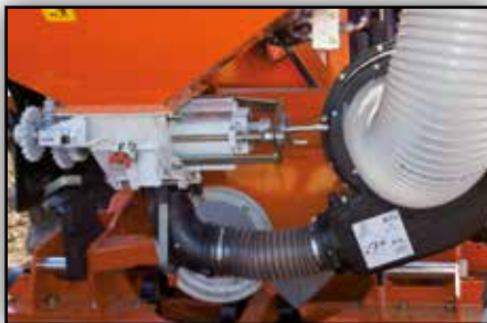
Adjustment of the metering device requires no tools
