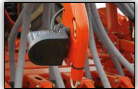
Always the right speed! A radar speed sensor records the speed in order to maintain the relevant distribution rate at the correct time.
