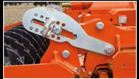
The depth adjustment bracket is positioned closer to the headstock to reduce stress on the whole construction and to allow the ease of fitment of all Kubota packer roller types.
