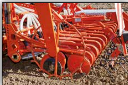
Landwheel with integrated brake to prevent overseeding, e.g. on headlands
