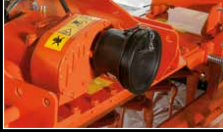
Robust change gear box with replaceable gears as standard. Additional sets of gears are available.
