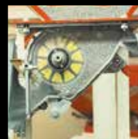
Setting for fine seeds, with rotary brush
