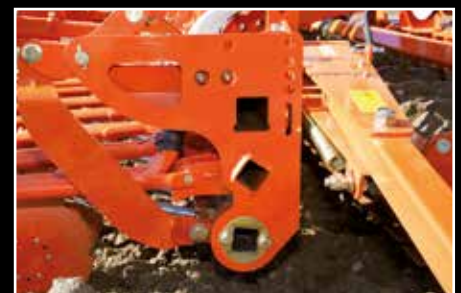
Overload protection of the marker arm
