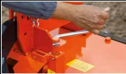
Spring loaded, infinite adjustment of the rear level-ling bar ensures a level surface.
