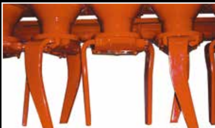
Fully welded rotor housings ensure high bending and torque resistance to the trough when working in very tough soil conditions. This also provides an optimum clearance between the trough bottom and tine holders and allows large amounts of residues and stones to pass freely without blocking.
