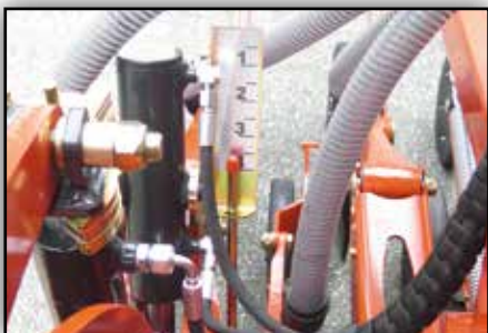
The sowing depth can be adjusted toolless by spacers which are located at the two outer hydraulic cylinders. The operator can see the coulter pressure setting on the scale which is easily visible from the tractor cab.
