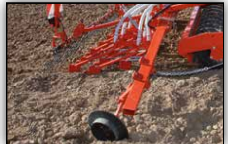
Exact continuation from one tramline to the next is ensured by the use of hydraulically folding track markers.
